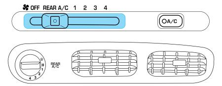
turn the Rear Fan Control on the main climate control system to Rear A/C and turn the Rear A/C Fan Control to 0.
